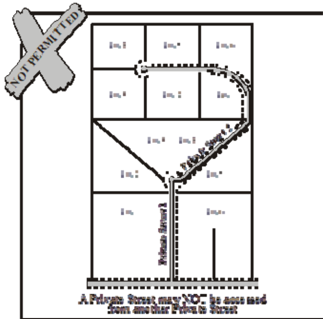
Figure 3.3 - Improper Use of a Private Street
